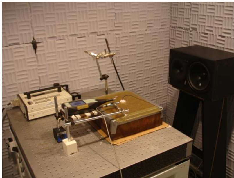
Fig. 5.8. Experimental setup for in vitro air-borne sensitivity experiments
